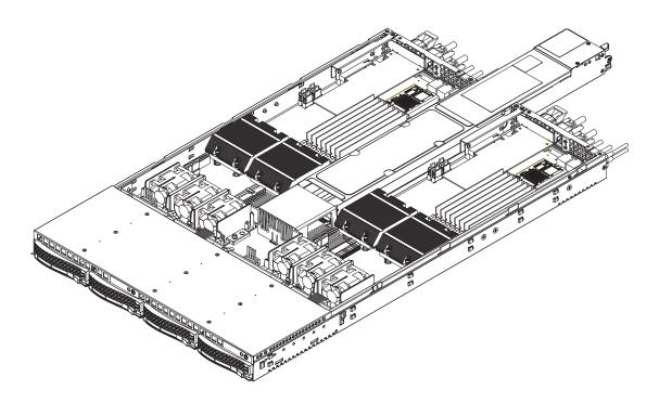
Figure 6-4. Removing the Power Supply
